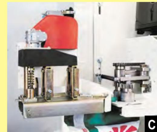
**Apply the hot-melt glue (B).** The hot-melt glue is applied using a hot-melt glue spraying device.
